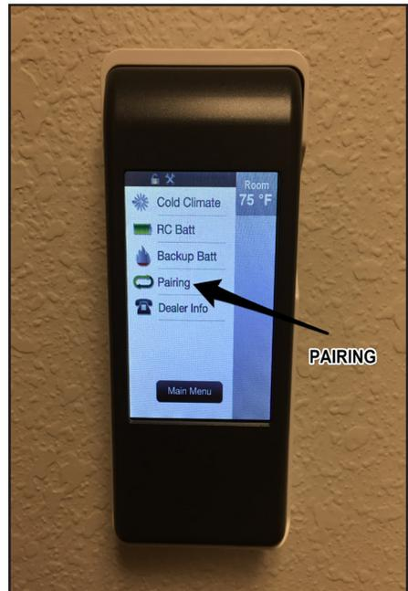
Figure 8. IFT-RC400 Wall Mount / Pairing Screen
