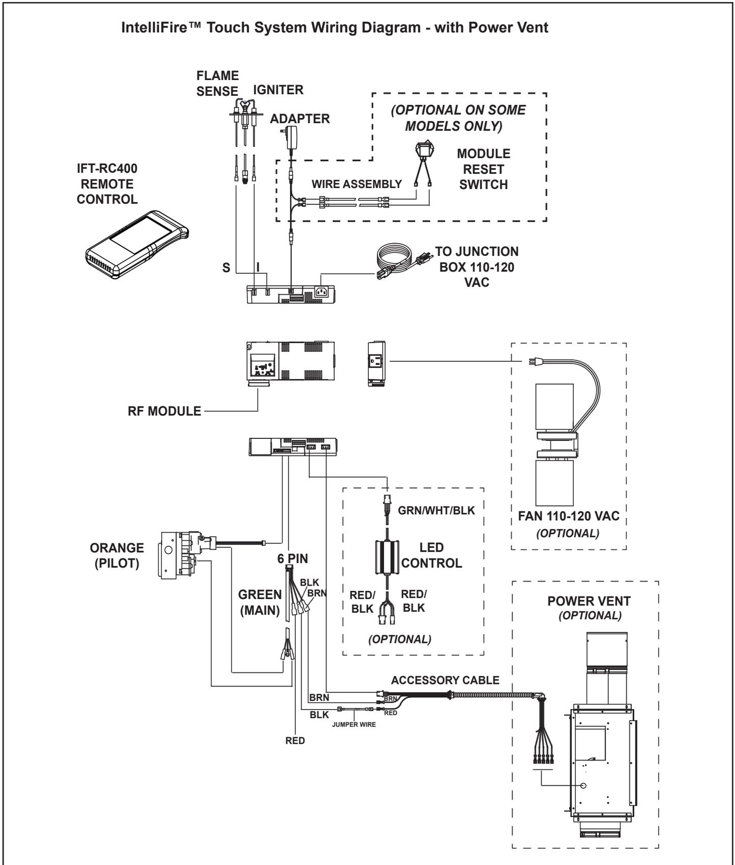
Figure 11. IFT-RC400 Wiring Diagram with Power Vent
