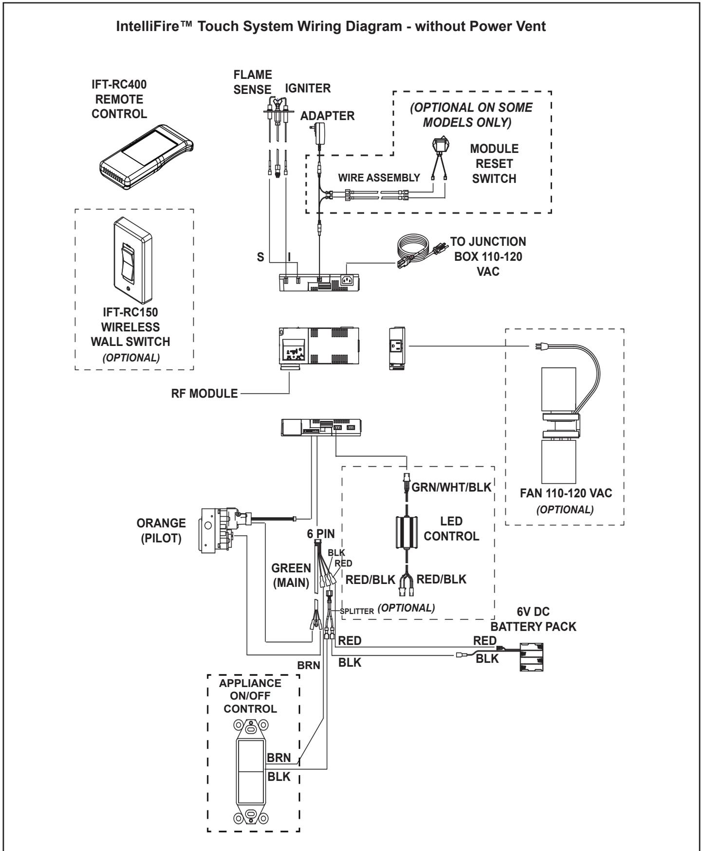
Figure 10. IFT-RC400 Wiring Diagram without Power Vent
