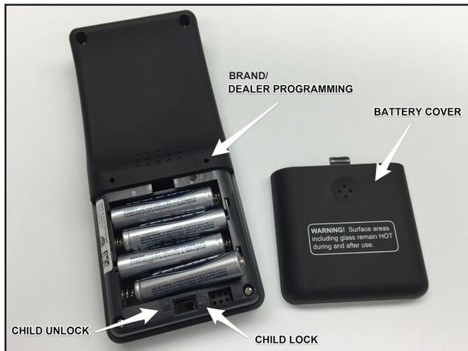
**Figure 5. Install Batteries & Child Safety**
