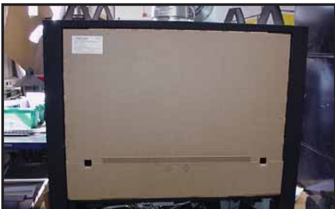
Figure 11.11 Splatter Guard with Lower Access Panel Open
