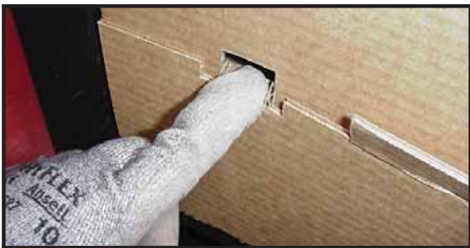
Figure 11.10 Securing Tabs Inside Front of Splatter Guard
