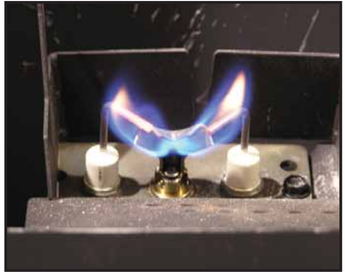
Figure 3.2 IPI Pilot Flame Patterns
