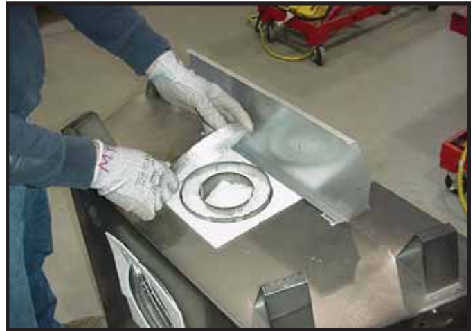
Figure 6.4 Remove the seal cap.
