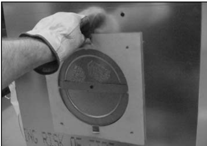
Schéma 7.7 Retirez le joint isolant
