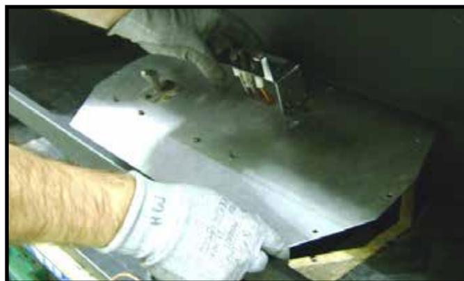
Figure 11.3. Retirer la plaque de vanne
