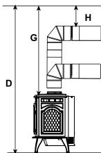
**Note:** Installation of optional blower does not affect minimum clearance dimensions, however, if frequent blower removal service is desired, clearance to the wall should be increased to  $B^*$  and  $C^*$  dimensions.
