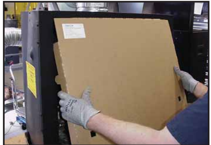
Figure 13.8 Installation of Splatter Guard
