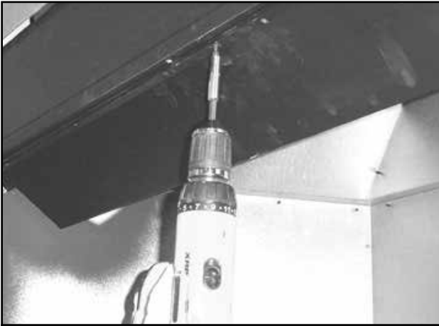
Figure 8.1 Remove Smoke Shield
