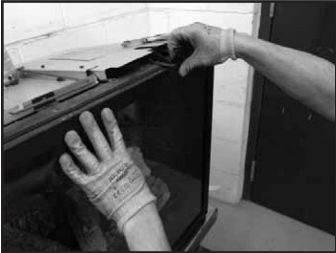
Figure 4.3 Release Glass Latches One at a Time
