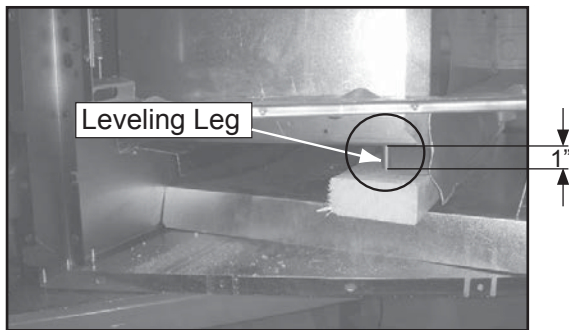
Figure 13.2. Ensure that the leveling leg is positioned over the 2 x 4 before leveling the insert. Minimum 1" clearance.
