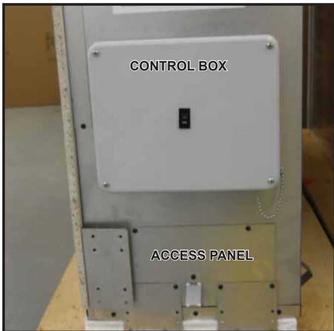
Figure 6.1 Control Box & Access Panel Locations
