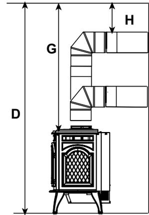
**Note:** Installation of optional blower does not affect minimum clearance dimensions, however, if frequent blower removal service is desired, clearance to the wall should be increased to B\* and C\* dimensions.
