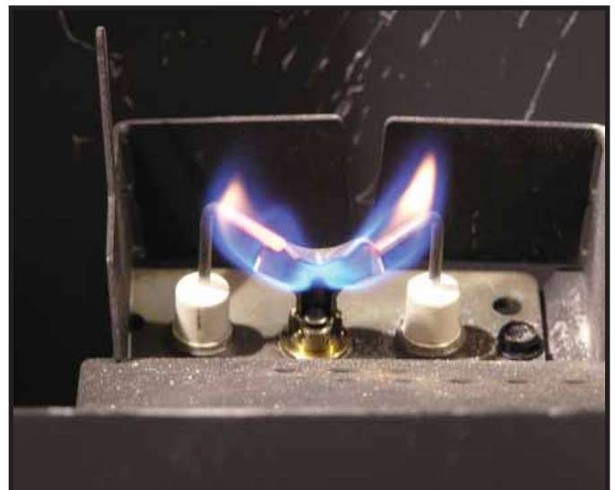
Figure 3.1 IPI Pilot Flame Pattern
