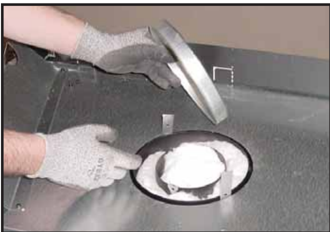
Figure 9.3 Remove the seal cap.
