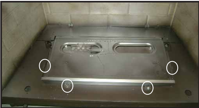
Figure 3.9 Remove Burner Skirt
