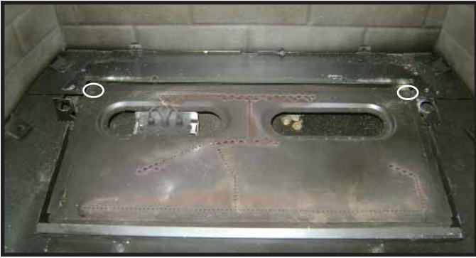
Figure 3.8 Remove Screws from Burner Assembly Rear Corners
